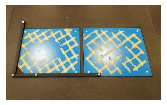
*Figure 7.* Calibration of the 3D coordinates in the space with an L-Frame.
