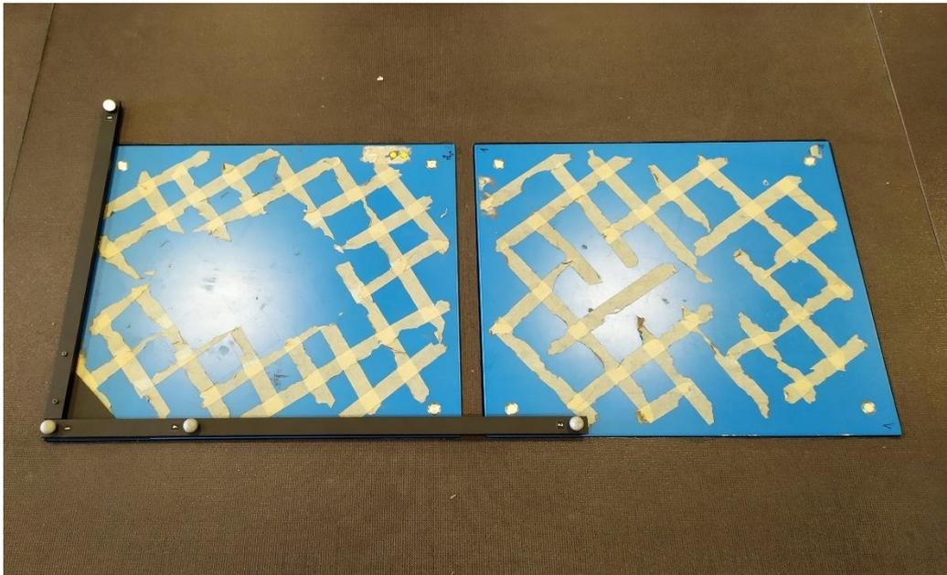
*Figure 7. Calibration of the 3D coordinates in the space with an L-Frame.*
