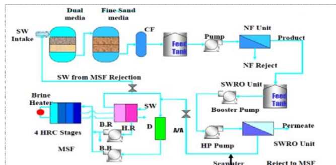
Figure 1.15. Working principle of a hybrid scheme of Nano-filtration/MSF/RO desalination unit [43]
