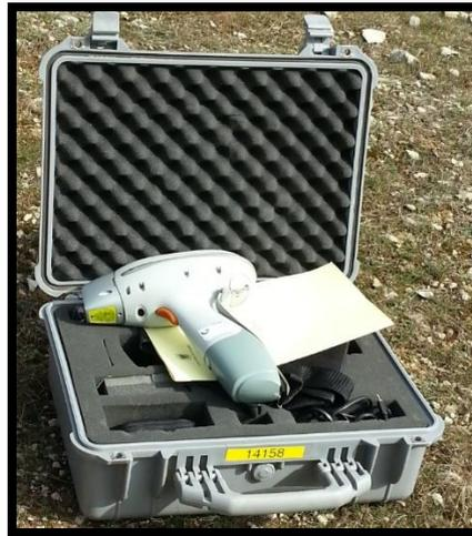
Figure m.6. NITON XLT 792 analyzer.
