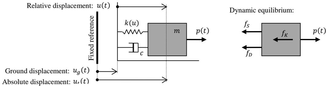
Fig. 1. SDOF system usually employed in earthquake engineering.
