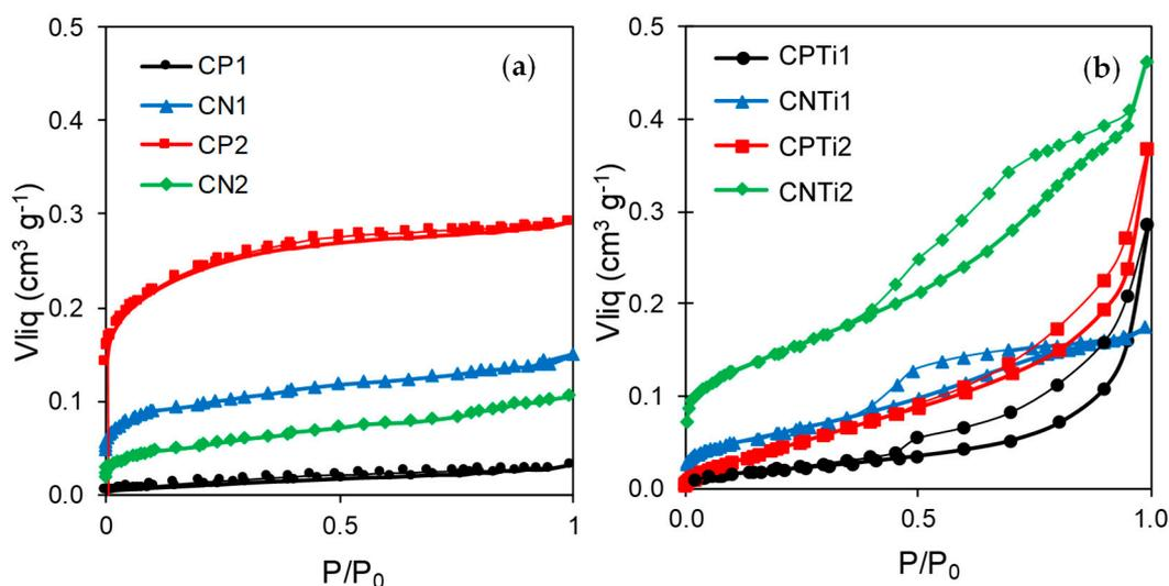
**Figure 6.** N<sub>2</sub> adsorption–desorption isotherms of (a) the pure carbon materials and (b) the carbon–Ti composites.
