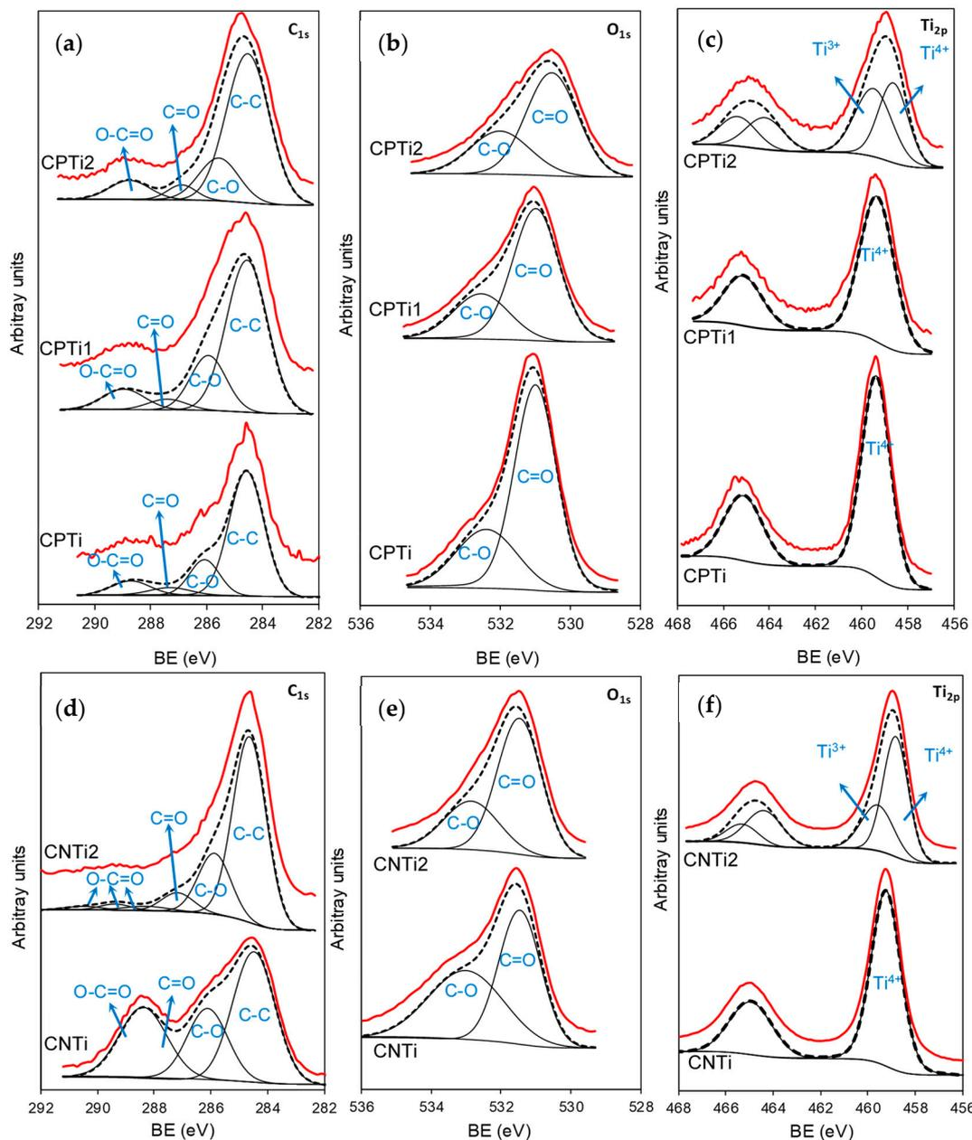
**Figure 2.** High-resolution XPS spectra of the C1s (a,d), O1s (b,e) and Ti2p (c,f) regions for Ti-impregnated cellulose derivatives and their corresponding carbonized composites.
