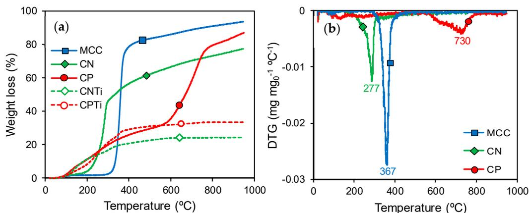
**Figure 1.** (a) Thermogravimetric (TG) profiles under N<sub>2</sub> flow for microcrystalline cellulose (MCC) and acid-treated cellulose samples before (solid lines) and after Ti impregnation (dash lines); (b) Differential thermogravimetric (DTG) profiles under N<sub>2</sub> flow for MCC, CN and CP.
