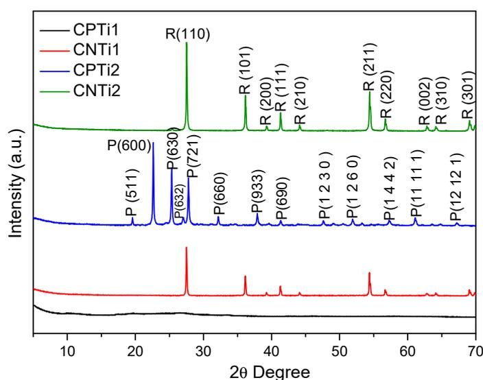
**Figure 3.** X-ray diffraction (XRD) patterns of the carbon–Ti composites (R = rutile, P = TiP<sub>2</sub>O<sub>7</sub>).
