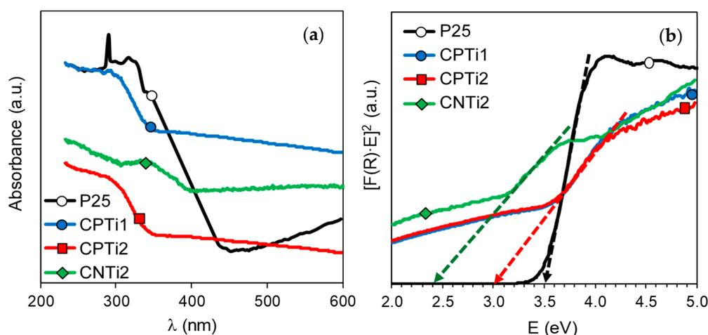
**Figure 7.** (a) UV/Vis diffuse reflectance spectra (DRUV) of P25 and different carbon–Ti composites. (b) Plot of transformed Kubelka–Munk units as a function of the energy of light (inset: determination of the band gap).
