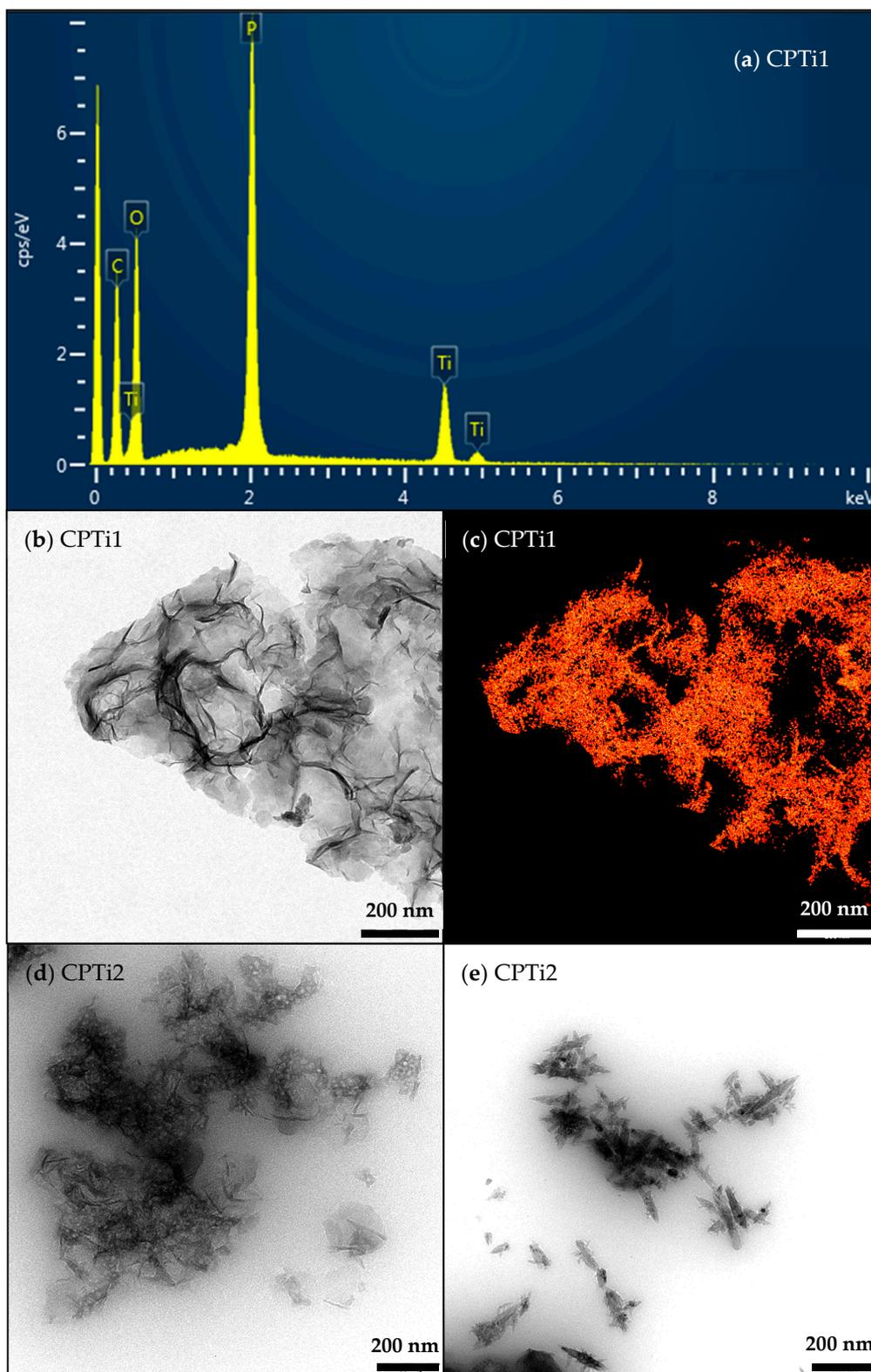
**Figure 5.** High resolution transmission electron microscopy (HRTEM) characterization of CPTi composites: (a) energy dispersive X-ray (EDX) analysis, (b,d,e) micrographs and (c) Ti-mapping.
