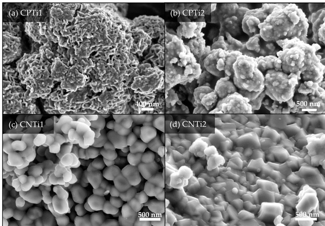
**Figure 4.** Scanning electron microscopy (SEM) images of the carbon–Ti composites prepared by cellulose treatment with phosphoric acid (a,b), or nitric acid (c,d).
