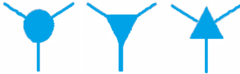
Fig 2.49 Geometries used to define the central conductor
