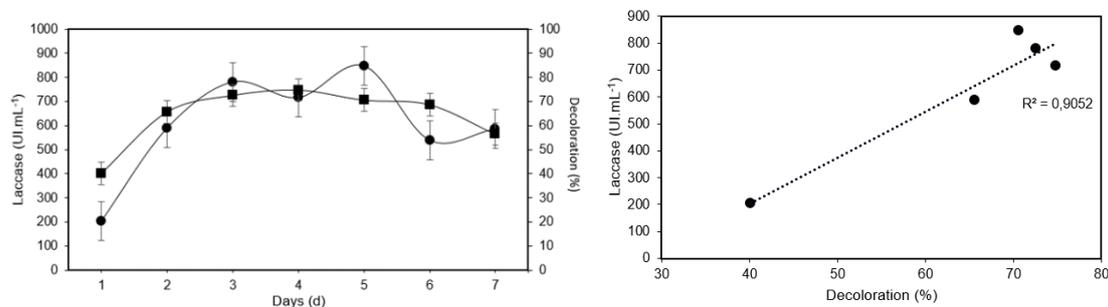
Figure 11. a) Time course of decoloration (■) and laccases production (●) in small scale inoculated with *G. lucidum* attached on peach palm residue. b) Relationship between the percentage of decoloration and laccase activity in a small scale.
