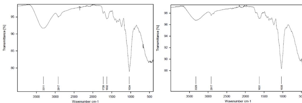
Figure 14. Bioreactor FTIR spectrometry. a) Time zero; b) after fifty days of cultivation.
