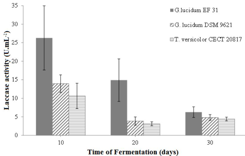
Figure 9. Time course in SSF experiments carried out with 40 mL of final effluent (100%) and three different WRF for Laccase activity.
