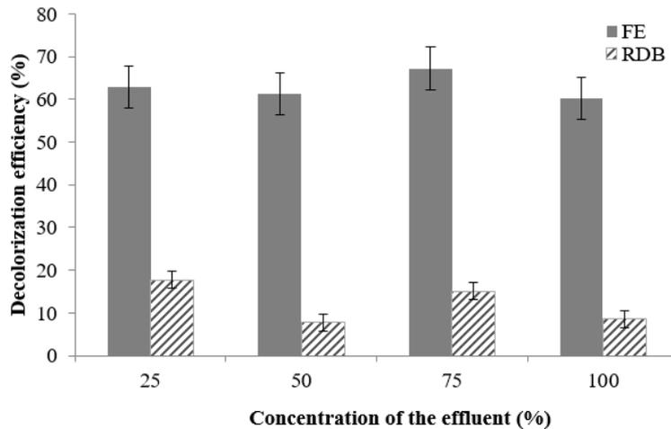
Figure 10. Decolorization efficiency obtained in the adsorption assays carried out with 60 mL of FE and RDB.
