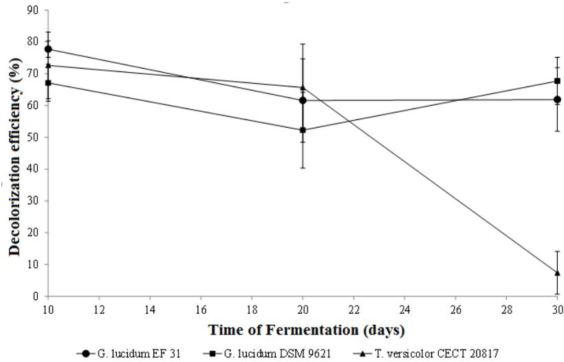
Figure 8. Time course in SSF experiments carried out with 40 mL of final effluent (100%) and three different WRF for decolorization efficiency<sup>-1</sup>).
