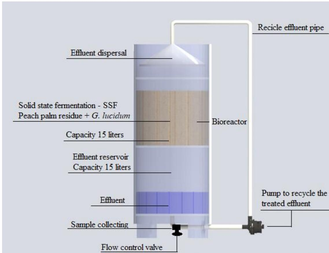
Figure 3. Schematic overview of the packed bed bioreactor.
