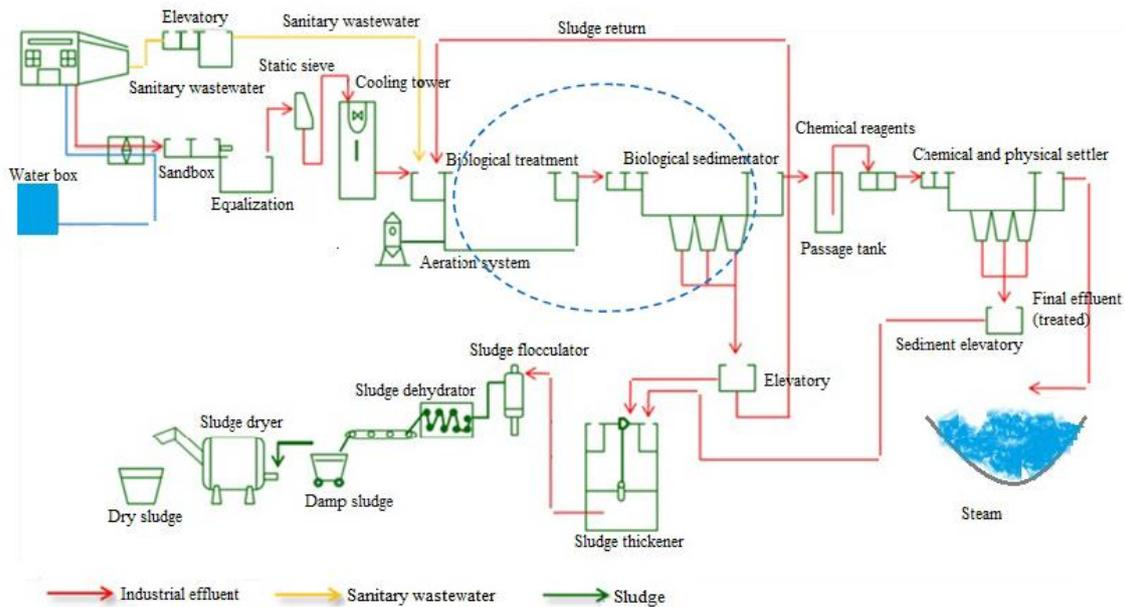
Figure 1. Diagram of effluent treatment plant using activated sludge, as show in the circle, typically used for the treatment of textile effluent.
