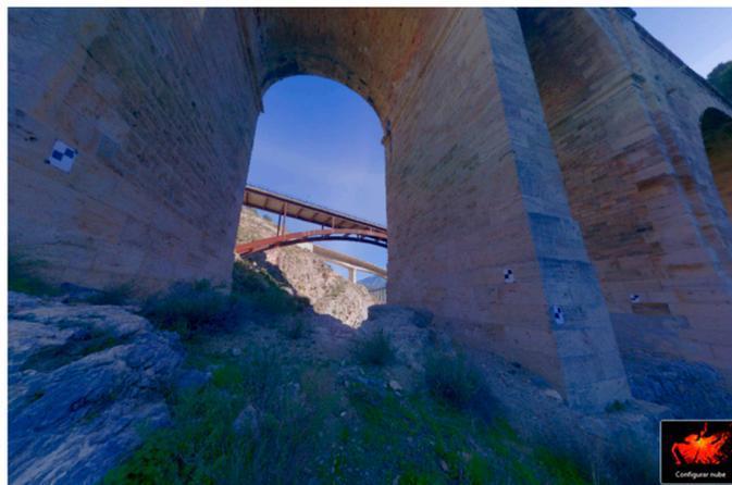
**Figure 7.** Targets used to register the BLK360 scan stations.
