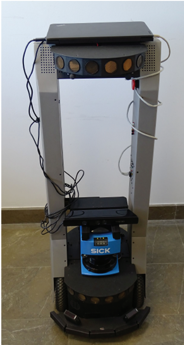
Figure 1 | Peoplebot robot equipped with laser rangefinder SICK LMS200 and a Kinect camera.
