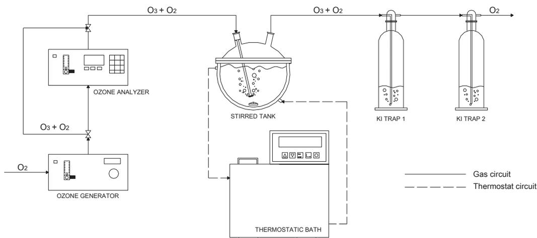
Fig. 2. Schematic diagram of the ozonation system
