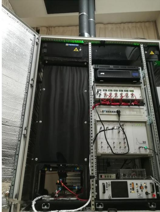
Figure III-3: Multiwavelength Raman lidar system.
