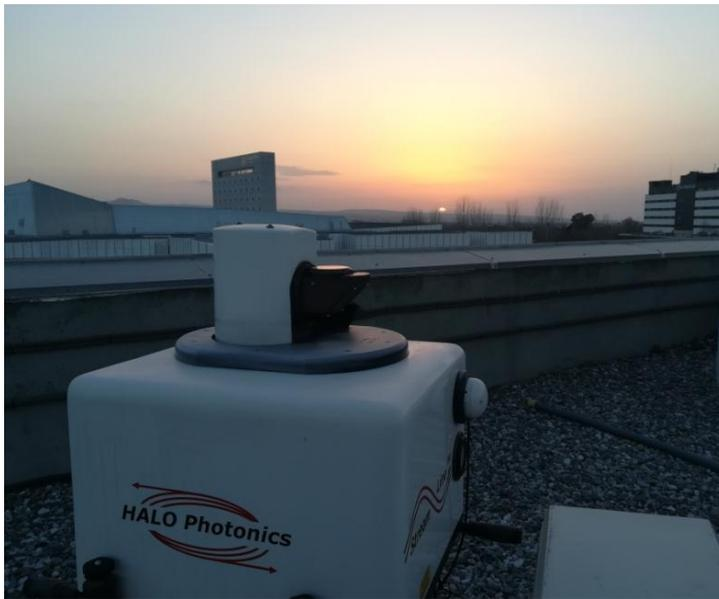
Figure III-5: Doppler lidar system on UGR station roof.
