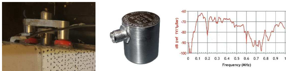
Figure 6.10. Attachment of the sensor R15 \alpha and its sensitivity curve.
