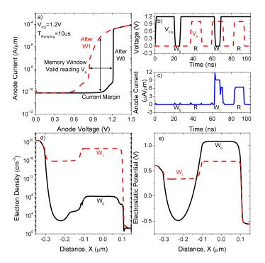
Fig. 2. a) Simulated  $I_A(V_A)$  curves after programming both states. b) Fast bias pattern and c) anode readout current for a W<sub>0</sub>-R-W<sub>1</sub>-R-W<sub>0</sub>-R memory operation applied to the default 200+200 nm Z<sup>2</sup>-FET device. d) Horizontal electron density profile and e) potential along the front-channel (1 nm away from top-interface) after programming the '1'- (W<sub>1</sub>, dashed line) and '0'-states (W<sub>0</sub>, solid line).  $V_{BG} = -1$  V and  $V_K = 0$  V.
