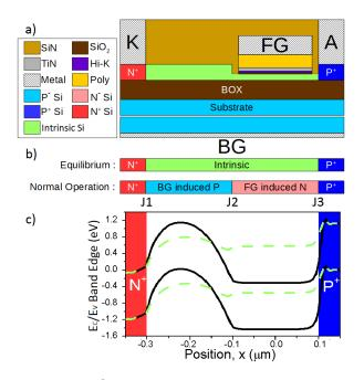
Fig. 1. a) N-type Z<sup>2</sup>-FET basic structure. b) Effective doping in *Si* active region at equilibrium ( $V_{FG} = V_{BG} = V_A = V_K = 0$  V) and in normal operation ( $V_{FG} > 0$  V and  $V_{BG} < 0$  V with  $V_A = V_K = 0$  V). c) Energy bands diagram at equilibrium (N<sup>+</sup>-I-P<sup>+</sup> diode, dashed line) and in normal memory operation (virtual N<sup>+</sup>-P-N-P<sup>+</sup>, solid line).
