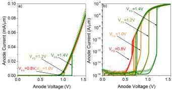
Fig. 3. Comparison of experimental data (symbols) with 2D simulations (solid lines).  $I_A(V_A)$  hysteresis curves in a) linear and b) log scale for several front-gate voltages.  $V_A$  is swept from 0 to 1.5 V and way back (triangular shape) with a 24.16 s ramp time for several front-gate voltages.  $L_G = L_{In} = 200$  nm,  $V_K = 0$  V and  $V_{BG} = -1$  V.
