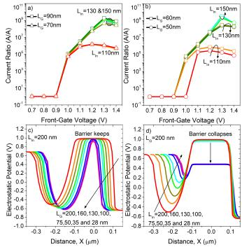
Fig. 5. a-b) Current ratio  $(I_1/I_0)$  against  $V_{FG}$  for different gate and intrinsic regions lengths. Simulated horizontal mid-channel potential when scaling c) the gate length or the d) intrinsic ungated region for 200, 160, 130, 100, 75, 50, 35 and 28 nm.  $V_{FG} = 1$  V,  $V_{BG} = -1$  V and  $V_A = V_K = 0$  V.
