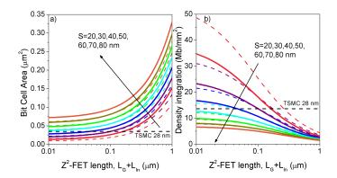
Fig. 10. a) Z<sup>2</sup>-FET bit cell area consumption and b) maximum density integration for different values of S as a function of the Z<sup>2</sup>-FET overall length  $(L_G + L_{In})$ . W = 100 nm (thick solid lines) and W = 60 nm (thinner dashed lines). Horizontal dashed line corresponds to the TSMC 28 nm eDRAM cell [15].  $L_S = 28$  nm and  $A_{Over} = 50$  %.
