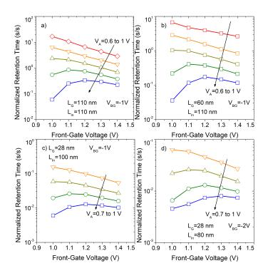
Fig. 8. Simulated retention time for scaled Z<sup>2</sup>-FETs: a)  $L_G/L_{In} = 110/110$  nm, b)  $L_G/L_{In} = 60/110$  nm, c)  $L_G/L_{In} = 28/100$  nm and d)  $L_G/L_{In} = 28/80$  nm.  $V_K = 0$  V.
