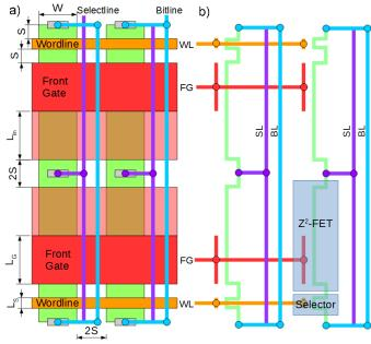
Fig. 9. Simplified diagram of a) possible layout and b) electrical connections for a 2x2 symmetric  $Z^2$ -FET memory matrix. Identical spacing between elements, *S*, is considered. Green colour: active silicon region; solid red:  $Z^2$ -FET front-gate; light red: intrinsic  $Z^2$ -FET region; orange: selector device front-gate acting as wordline; purple: select line; light blue: bitline.
