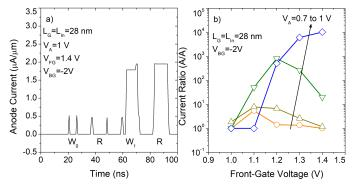
Fig. 7. a) Memory operation and b) current ratio of Z<sup>2</sup>-FET cell scaled beyond 28 FD-SOI technology:  $t_{Si} = 4.8$  nm,  $t_{BOX} = 15$  nm,  $N_{In} = 10^{17}$  cm<sup>-3</sup> and no silicon epitaxy.  $V_K = 0$  V.
