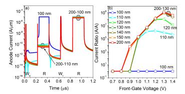
Fig. 4. a) Current readout at  $V_{FG} = 1$  V for a W<sub>0</sub> ( $V_A = 1$  V and  $V_{FG} = 0$  V), R ( $V_A = 1$  V and  $V_{FG} = 1$  V), W<sub>1</sub> ( $V_A = V_{FG} = 0$  V), R bias pattern. b) Current ratio ( $I_1/I_0$ ) for different lengths.  $V_K = 0$  V and  $V_{BG} = -1$  V. Programming and reading last 5 ns and 200 ns, respectively.
