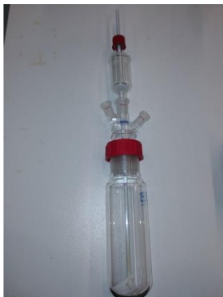
Figure 39. 90 mL reactor for the synthesis of amino-functionalised cross-linked polystyrene NPs.
