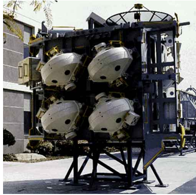
Figure 1: Control moment gyroscope installed in the International Space Station [25]
