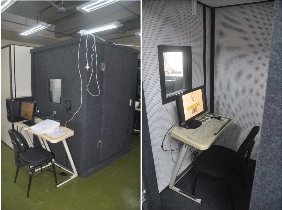
Figure 1.2. Sound-attenuation chamber where data were collected in Experiments 1 and 2. The computer and monitoring screen were set outside the cabin (left). Inside, the participant tried to control the lamp bulb which appeared 50 times on the screen using the keyboard, and made self-assessments with the mouse (right).
