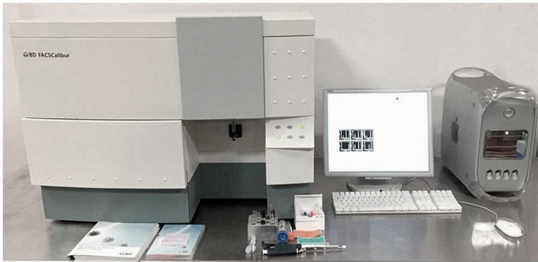
Figure 1.13. BD FACScalibur TM 2 Laser, 4 Color Flow Cytometer (Becton Dickinson). (Picture obtained from BD Biosciences, USA).
