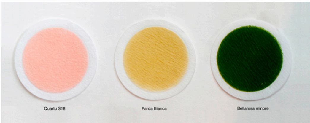
Figure 1.12. Particles concentrated on 0.7 \mu\text{m} pore-size Whatman GF/F glass fiber filters from different study ponds in Molentargius (Sardinia).
