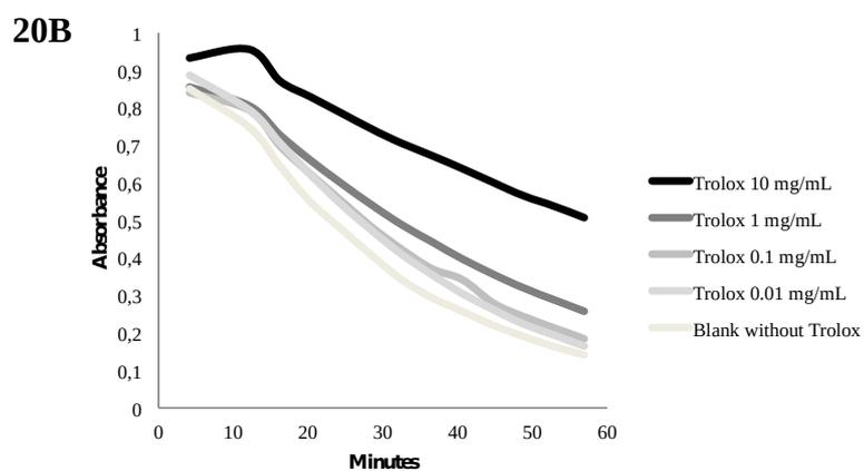
**Figure 21.** Absorbance spectra of catechin and Trolox (21A) and kinetics curves of Trolox (21B) as standard (iron 100  $\mu$ M, phosphotungstate 100  $\mu$ M, H<sub>2</sub>O<sub>2</sub> 4M, phosphate buffer 0.5M and carmine indigo 1 mM).
