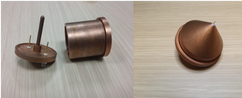
Figure 4.11: Different fabricated coaxial cavity resonators.
