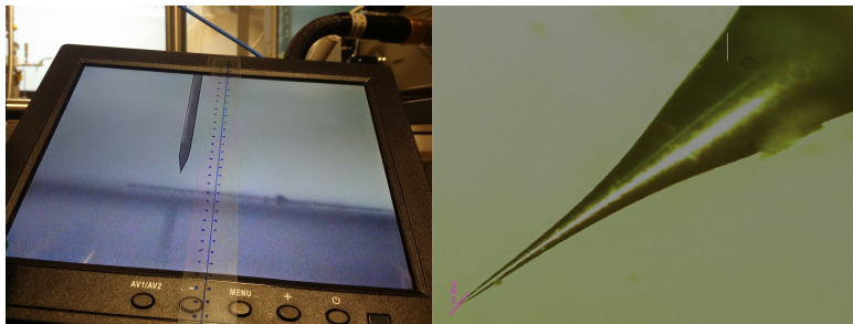
Figure 4.17: Tip used on the calibration of the NSMM system and the characterization of samples. In the left side, the cavity is connected to the probe tip with l = 1.7\text{mm} of length and d = 1.8\mu\text{m} in diameter. On the right side the tip connected to the cavity above the sample under test, using a LCD camera to capture a picture of the distance between tip-sample.
