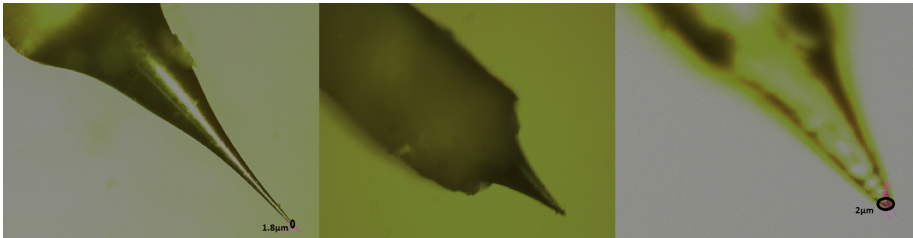
Figure 4.6: Different shapes of the tungsten wire during the etching automatically (Using a DC circuit and a tip mechanism holder).
