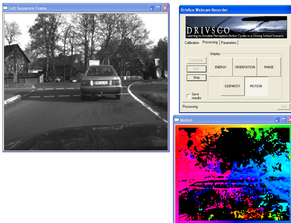
Figure 4.3: Screen capture of the optical flow application. - The optical-flow computation in real-time for the left input camera is displayed in the lower right screen.
