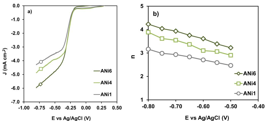
Figure 10. (a) LSV curves at 2500 rpm, and (b) variation of  $n$  with E vs. Ag/AgCl for samples ANi1 (○), ANi4 (□), ANi6 (◇).
