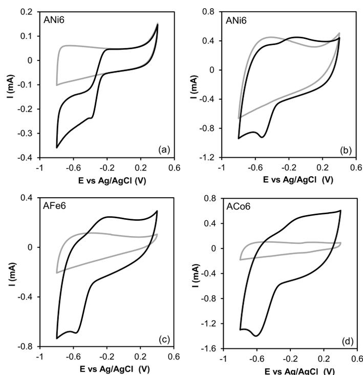
**Figure 8.** Cyclic voltammeteries on  $\text{N}_2$ -saturated  $\text{KOH}$  0.1 M (grey) and  $\text{O}_2$ -saturated  $\text{KOH}$  0.1 M (black). (a)  $5 \text{ mV}\cdot\text{s}^{-1}$ ; (b–d)  $50 \text{ mV}\cdot\text{s}^{-1}$ .
