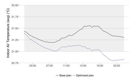
**Figure 3.** Indoor temperature values (average) of the base and the optimized operational plans obtained after simulation in the intermediate day (6 February 2017) (the comfort range [21, 22] is highlighted).
