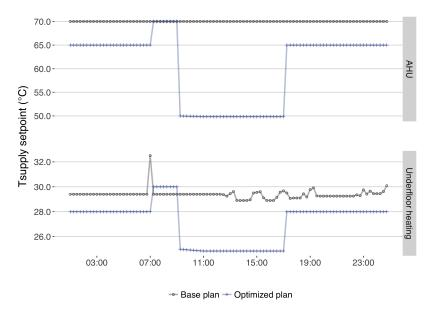
**Figure 2.** Temperature supply setpoint values of the base and the optimized operational plans simulated in the intermediate day (6 February 2017).
