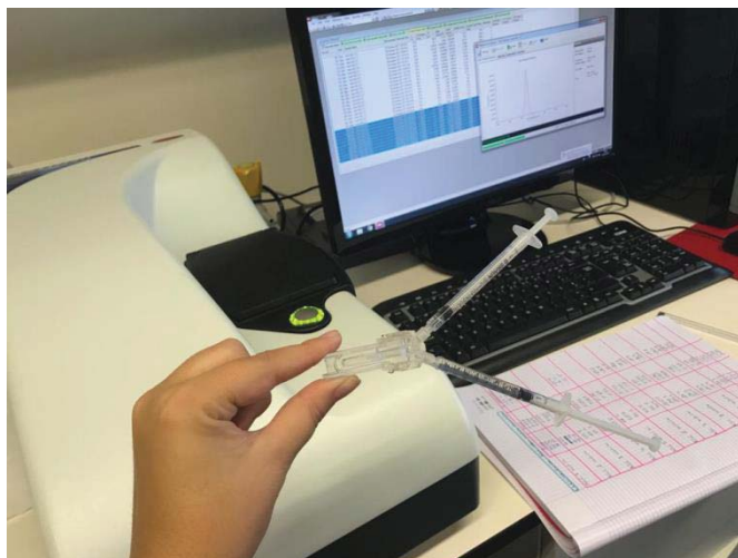
Figure 26. Sample cell for zeta potential measurement
