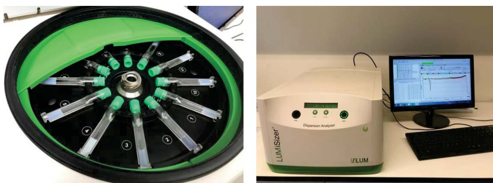
Figure 28. LUMiSizer equipment and cuvettes-type analytical centrifugation
