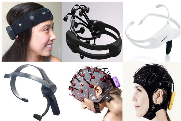
Figure 2.2: Commercial low-cost wireless EEG acquisition systems. From top left to bottom right: EEG headband (Cognionics), EPOC (Emotiv), Insight (Emotiv), MindWave (Neurosky), g.Nautilus (g.tec) and Enobio (Neuroelectrics).
