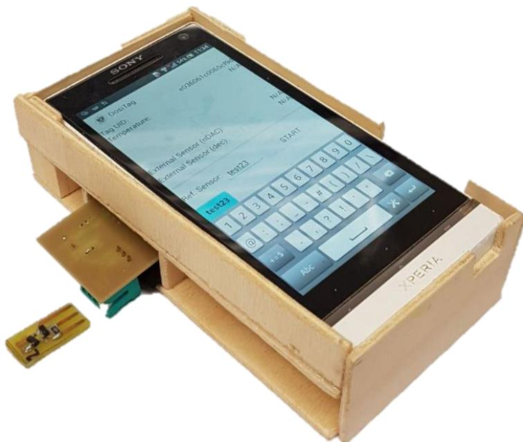
**Figure 69.** Experimental setup for NFC measurements using a custom-made wood structure to ensure adequate and repeatable inductive coupling.
