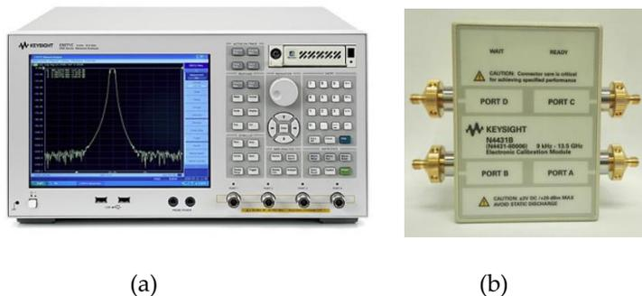
**Figure 30.** (a) RF Network Analyzer ENA model E5071C from Keysight Technologies and (b) N4431B RF Electronic Calibration Module (ECal).
