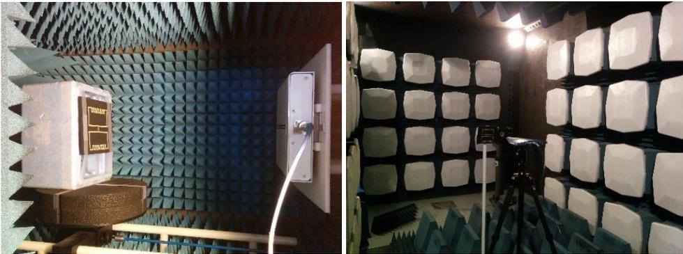
**Figure 51.** Measurements conducted inside the anechoic chamber using the Voyantic Tagformance System.
