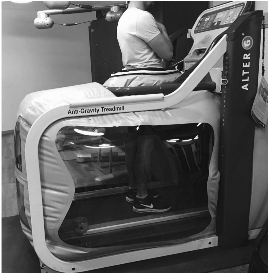
Figura 14. An illustrated example: Anti-gravity treadmill with the OptoGait system placed on the side edges at the same level as the contact surface
