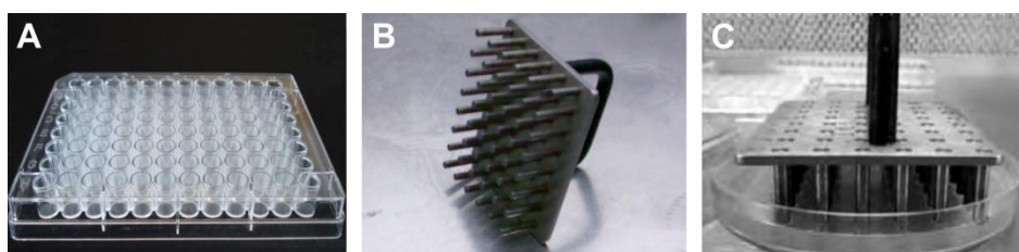
Figure M12. System used for the application of serial dilutions of liquid yeast cultures in Petri dishes to measure growth (drop-test assay). A) 96 well ELISA plate. B) Floating-pin replicator, containing 48 pins of 3.18 mm diameter. C) Application of serial dilutions of liquid yeast cultures in a Petri dish with the floating-pin replicator.
