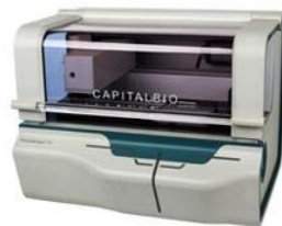
Figure 76: PersonalArrayer™16 (CapitalBio Corporation, China) used for the automatic spotting.
