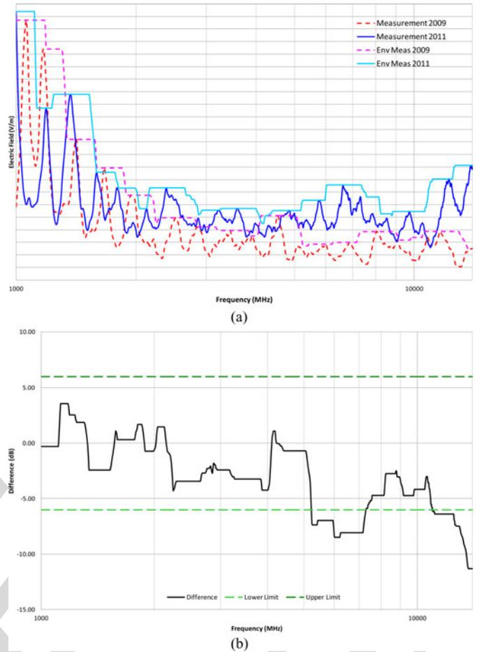
Fig. 12. (a) Comparison between two measurements on a point in the C-295 cockpit from different test campaigns. (b) Difference between the two measurements and 6 dB limit.
