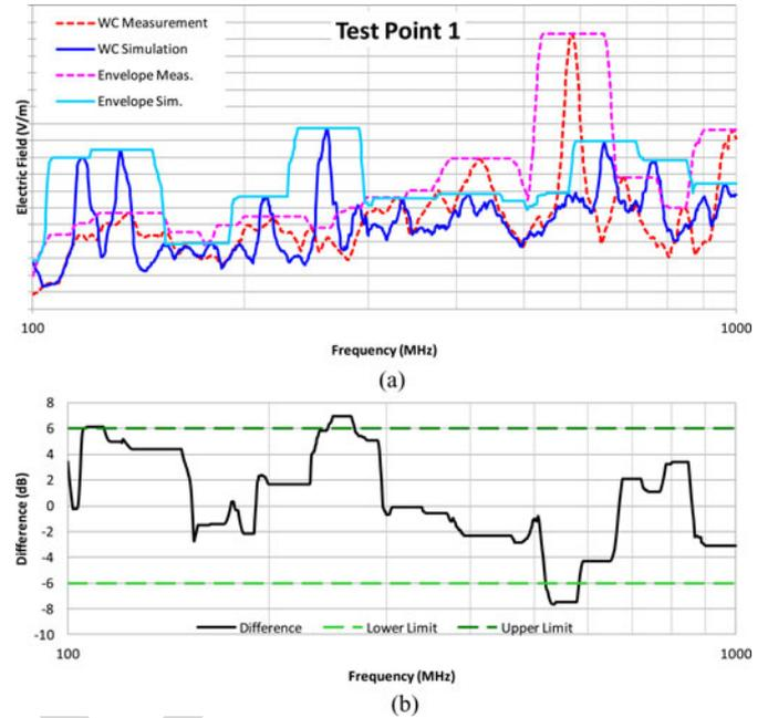
Fig. 6. (a) Comparison between measurements and simulations for the test point 1 located in the cockpit. (b) Difference between simulation and measurement and 6 dB limit.
