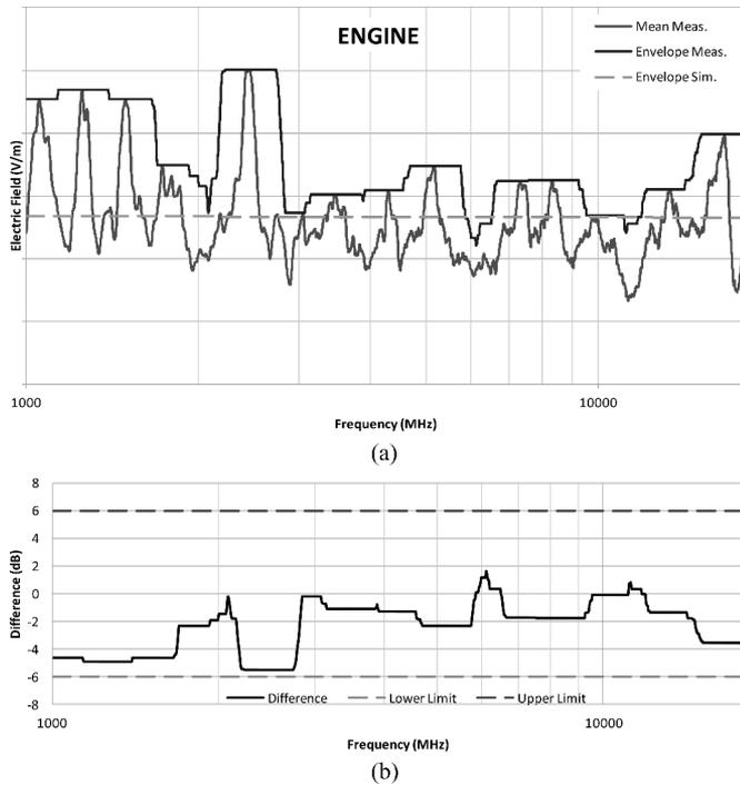
Fig. 11. (a) Comparison between measurements and simulations for the Engine. (b) Difference between simulation and measurement and 6 dB limit.
