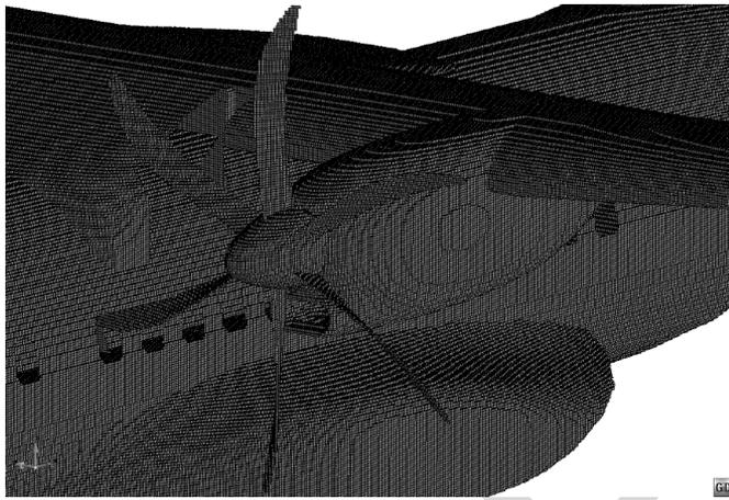
Fig. 5. Cartesian mesh of the engine and central fuselage external geometry.
