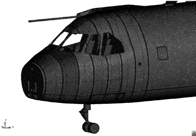
Fig. 4. C-295 cockpit unstructured mesh.
