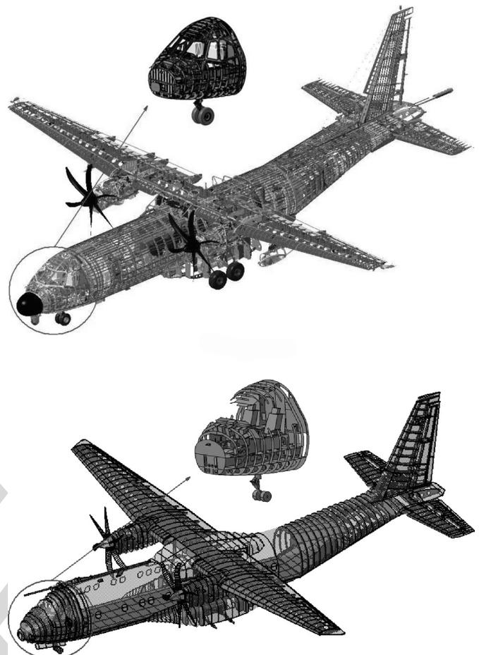
Fig. 3. (a) Isometric view of the C-295 digital mock-up with a detailed view of the cockpit. (b) C-295 simplified geometry with a detailed view of the cockpit (aerodynamic surfaces are depicted with a degree of transparency to allow the observation of the internal surfaces).
