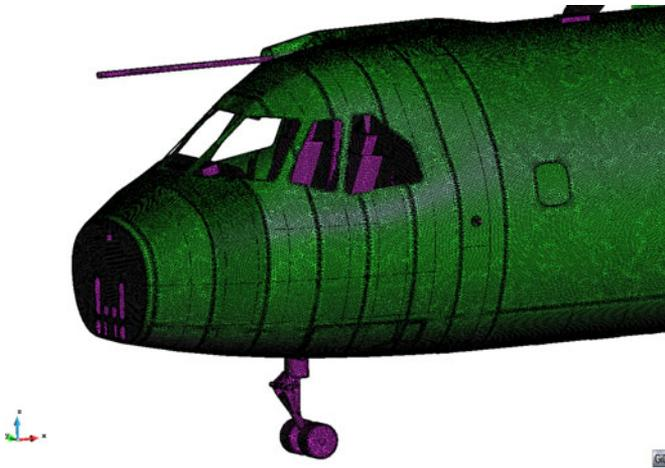
Fig. 4. C-295 cockpit unstructured mesh.
