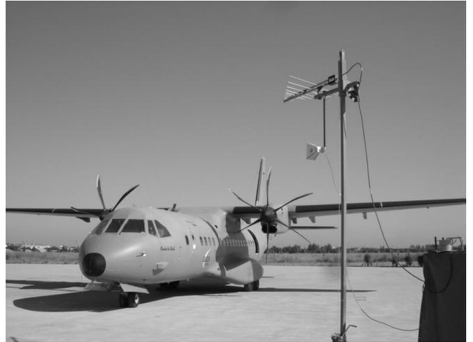
Fig. 1. LLSF tests at airbus military open-area test-site facility.
