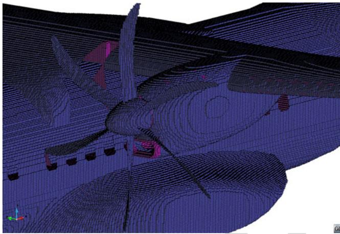
Fig. 5. Cartesian mesh of the engine and central fuselage external geometry.
