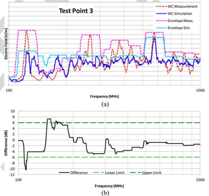
Fig. 7. (a) Comparison between measurements and simulations for the test point 3 located in the cargo bay. (b) Difference between simulation and measurement and 6 dB limit.
