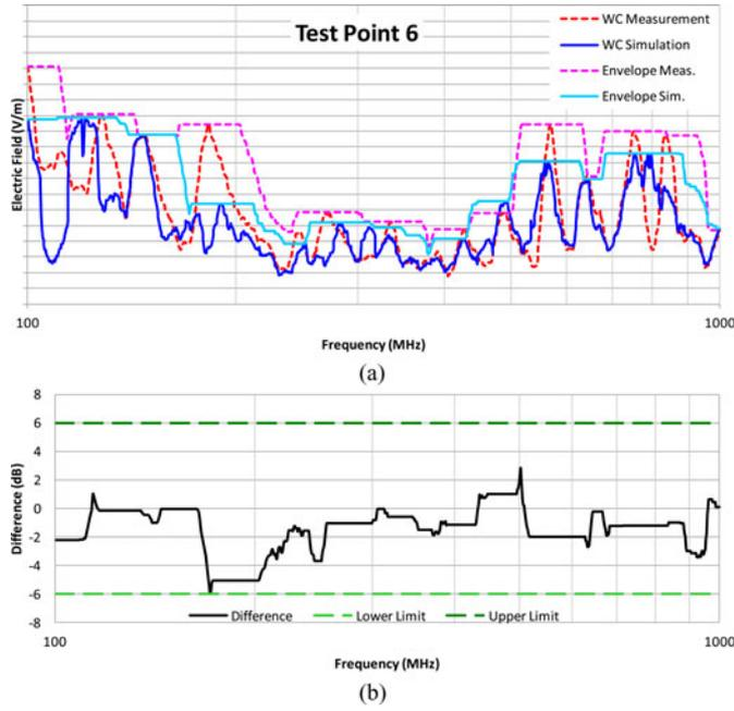
Fig. 8. (a) Comparison between measurements and simulations for the test point 6 located in the engine. (b) Difference between simulation and measurement and 6 dB limit.
