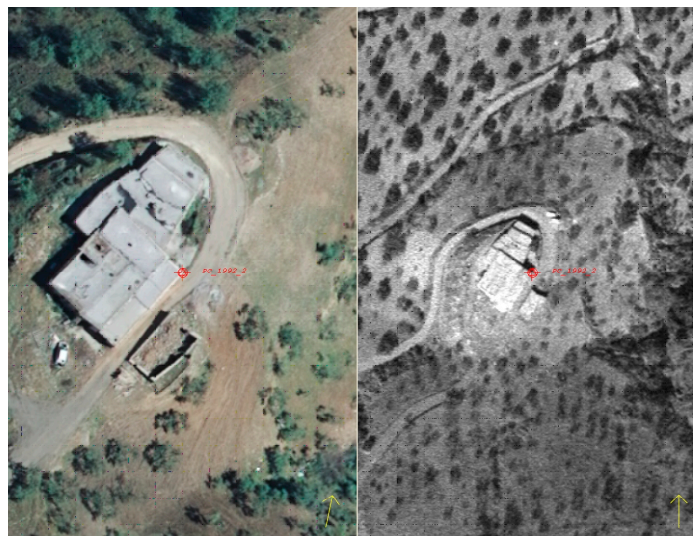
Figure 6. Example of transferred second-order control point (GCP).
