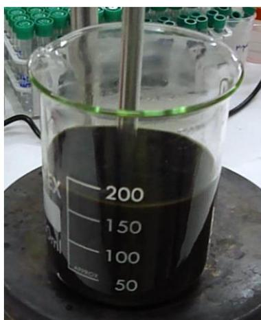
Figure 1.1: Dispersion of naphthenic bitumen in water at pH 12.
