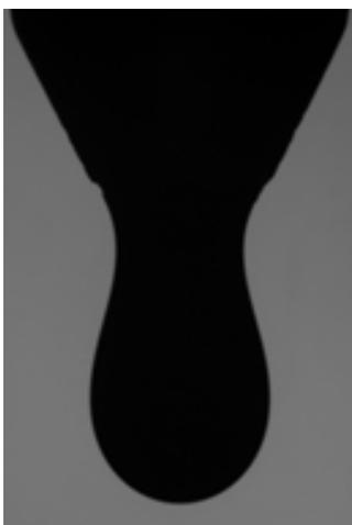
Figure 1.3: Bitumen pendant drop formed at high temperatures.
