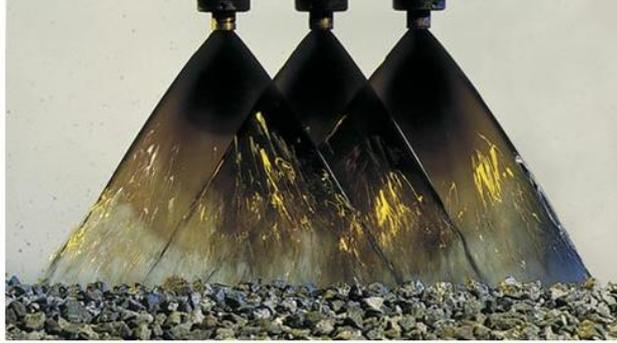
Figure 2: Application of bituminous slurry on mineral aggregates.
