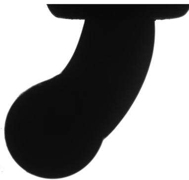
Figure A.3: Evidence of the elasticity loss of aged naphthenic bitumen. It is clear the spherical tip of the filament adopted after days from the dispensation.
