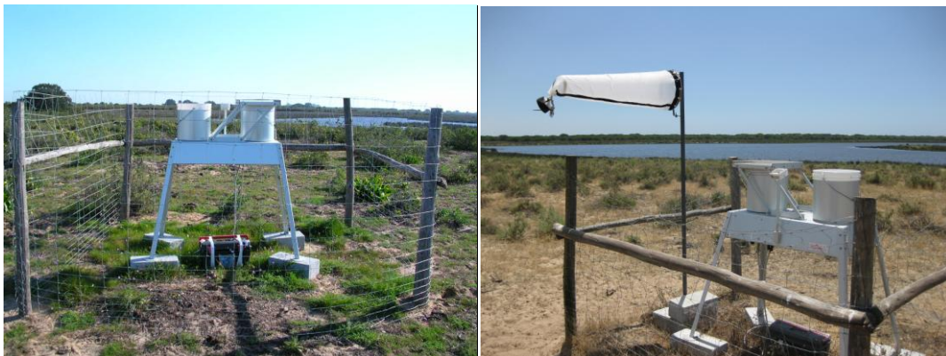
Figure 9. Automatic dry/wet atmospheric collectors and windsock (right) built in Doñana.
