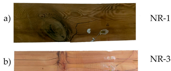
Figure 6. Breakage patterns of the NR beams group: (a) NR-1; and (b) NR-3.
