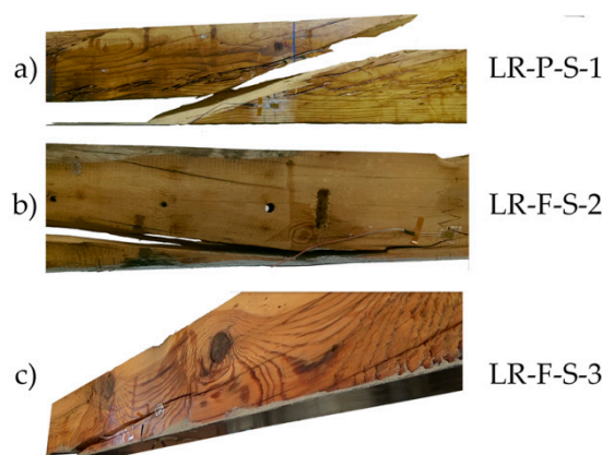
Figure 9. Breakage patterns of the LR beams group: (a) LR-P-S-1; (b) LR-F-S-2; and (c) LR-F-S-3. CFRP supplier: SIKA®.
