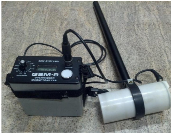
Fig. 4.2 Magnetometer GSM-8 used to obtain magnetic data.
