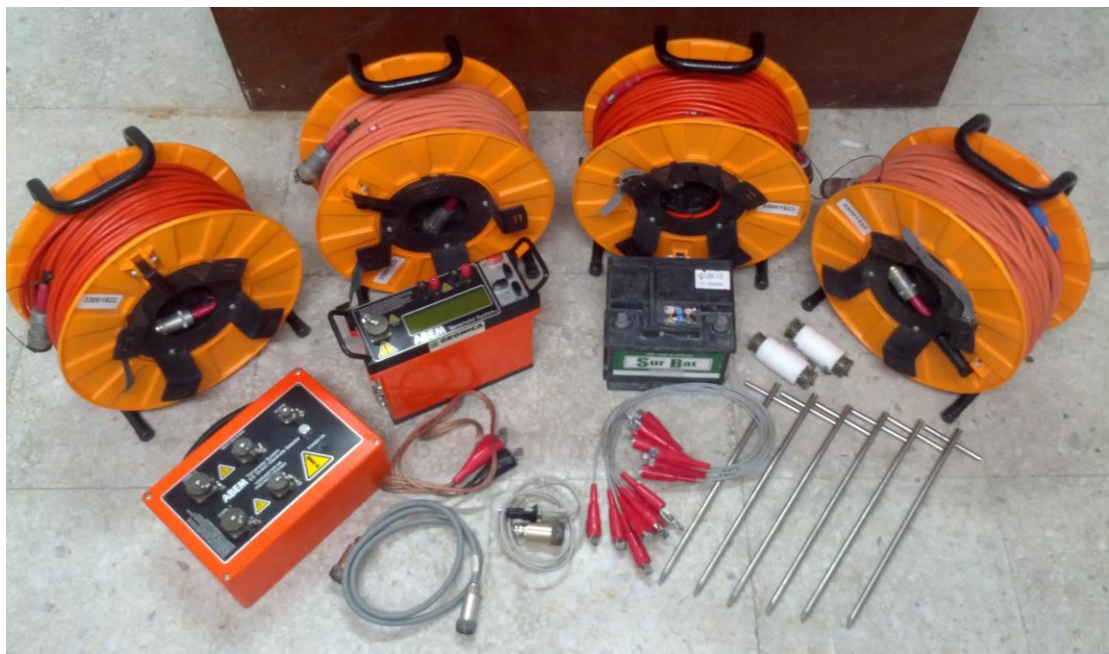
Fig. 4.3 Terrameter SAS 4000 used to obtain ERT profiles.
