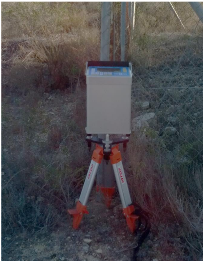
Fig. 4.1 Gravimeter Scintrex CG-5 AutoGrav used to acquire gravity data.
