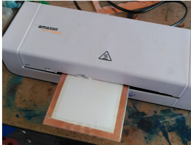
Figure D.2 – Transferring the stencil to the PCB
