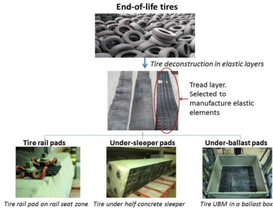
Figure 57. Elastic elements for railway high-speed from deconstructed end-of-life tires (without grinding up the material) (Sol-Sanchez et al., 2014).
