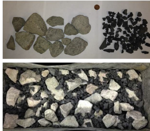
Figure 60. Visual appearance of the ballast and crumb rubber used as well as the mix of both materials (Sol Sanchez et al., 2015).
