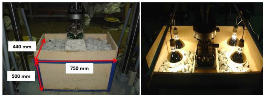
Fig. 1. Visual appearance of the full-scale test developed in a laboratory box.
