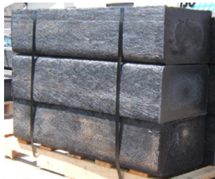
Figure 59. Railroad sleeper made of a rubber-plastic composite (Evans and Evans, 2006).
