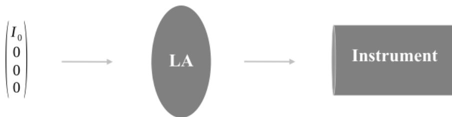
Figure 4.14: A linear polarizer placed between the light source and the instrument as a calibration unit in linear-polarization-only mode.
