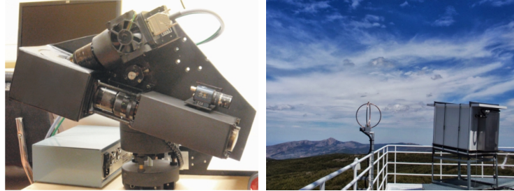
Figure 6.7: GRASSP instrument 0.23 nm resolution spectrograph (left) and housing together with a lightning detector (right) on the terrace of the 2.2 m dome of CAHA Observatory
