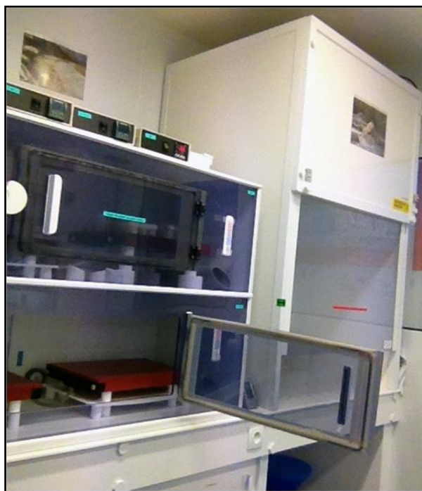
Figure 3.4 Hot-plate for sample dissolution and open beaker dry-down in closed system evaporation cabinets at the clean lab facilities in Géosciences Montpellier.
