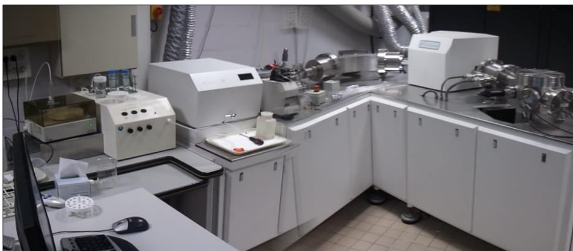
Figure 3.7 Nu Plasma 500™ MC-ICP-MS at the ENS of Lyon (France).
