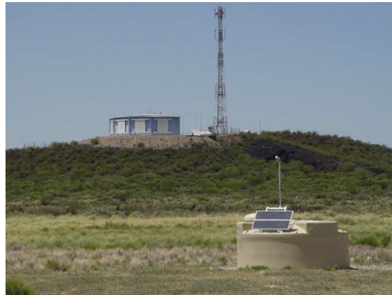
Figura 2.2: A fluorescence telescope enclosure, seen on the hill top, and a surface detector station, below.
