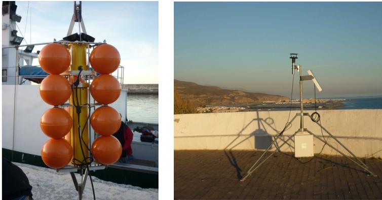
*Figure C.1: Photographs of the instruments used in the first field study. Left panel: structure of the ADP deployed on the bottom of the submarine canyon. Right panel: meteorological station located at the Sacratif Cape.*
