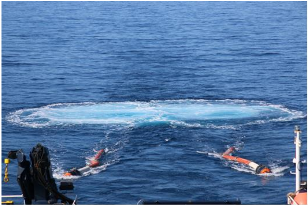
Figure 3.9. A picture of the real bubble generated by the air-guns mounted in the Vessel “Sarmiento de Gamboa”.
