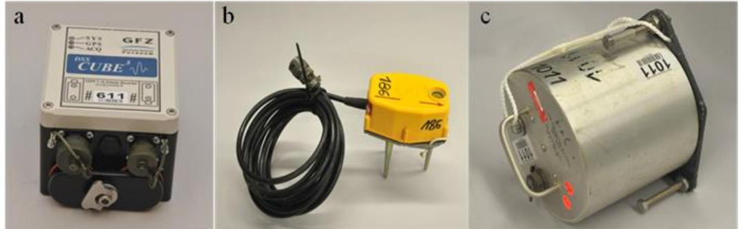
Figure 3.2. Pictures of the short-period seismic stations deployed on-land during the experiment and belonging to the GIPP (Germany). a) DATA-CUBE3 recorder, b) 3-D PE-6/B Geophone, c) Mark L4C sensors.
