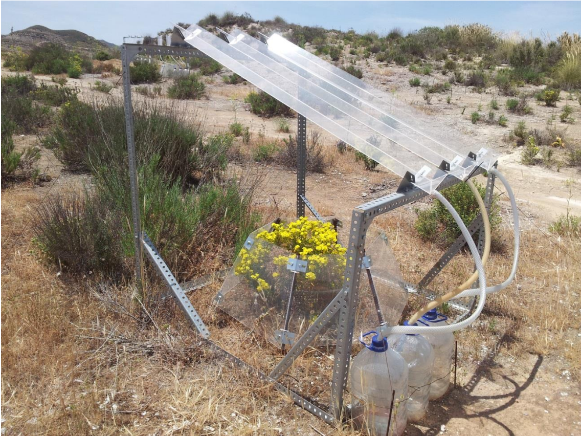
Figure 1. Experimental plot of the Warming + Rainfall Reduction treatment, which is achieved by installing an open top chamber (OTC) and a rainout shelter on the same plot.
