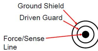
Figure B.7. Conductors inside a triaxial cable.
