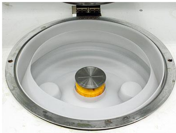
Figure C.4. The sample was placed in a vacuum spindle to carry out the application of the resist.
