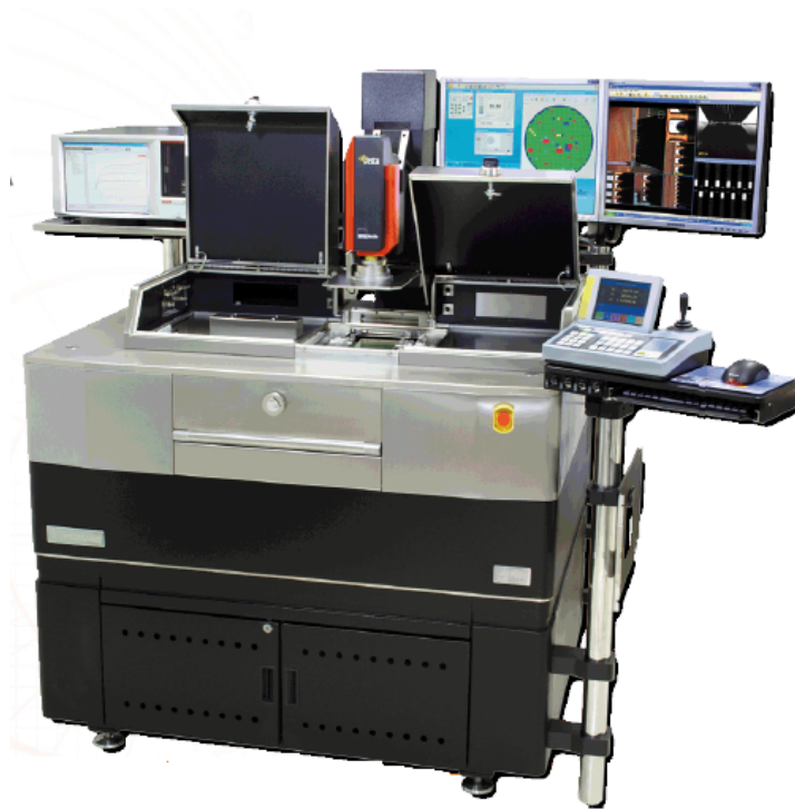
Figure B.14. Semi-automatic probe system by Suss Microtec. This equipment provides a perfect environment for an accurate wafer current and capacitance low-noise measurements.
