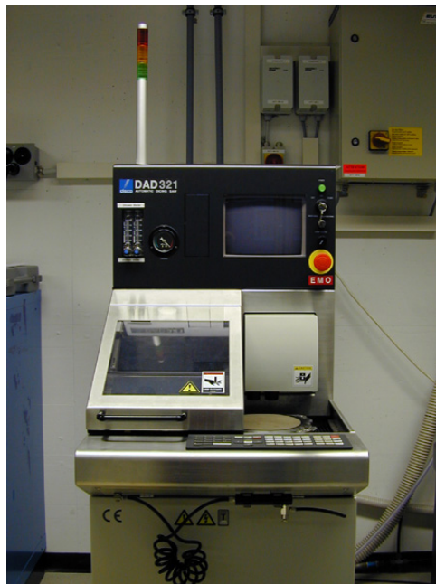
Figure C.2. Dicing saw (Disco DAD 321 machine) used to cut the substrate in smaller samples.
