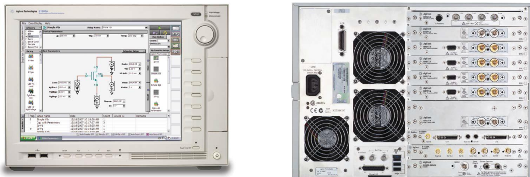
Figure B.2. Front and back view of the Agilent B1500A Semiconductor Analyzer.
