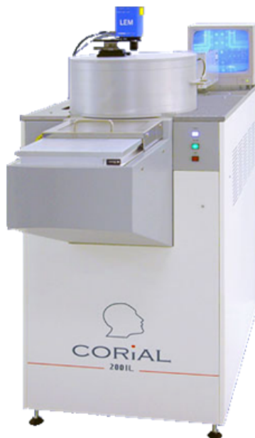
Figure C.8. The inductively coupled plasma etcher employed during the fabrication process.
