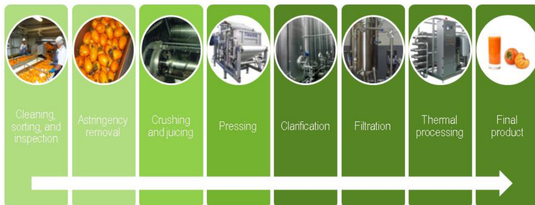
Figure 27. Basic scheme for fruit-juice production.
