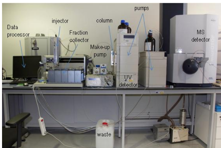
Figure 19. Semi-preparative HPLC equipment coupled to a ESI-TOF Mass Spectrometer.
