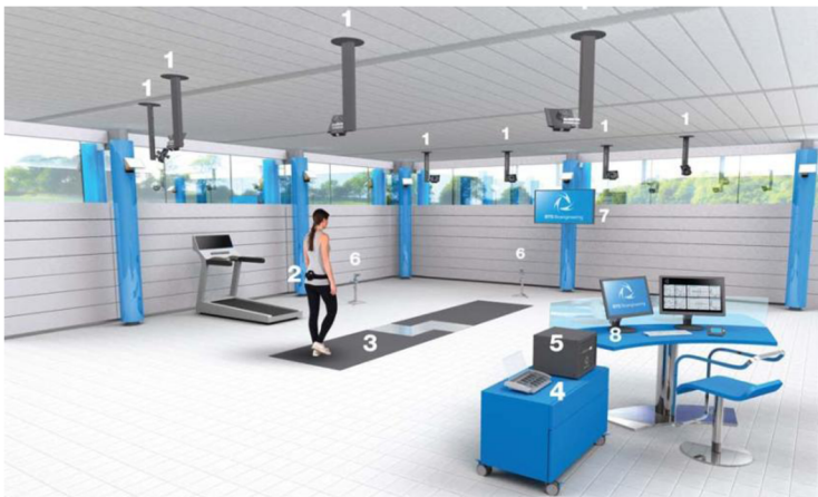
Figure 1.13: Example of non wearable system: BTS GaitLab configuration. (1) infrared videocameras; (2) inertial sensor; (3) GRF measurement walkway; (4) wireless EMG ; (5) workstation; (6) video recording system; (7) TV screen; (8) control station. Reproduced with permission from BTS Bioingeniering[53, 54].
