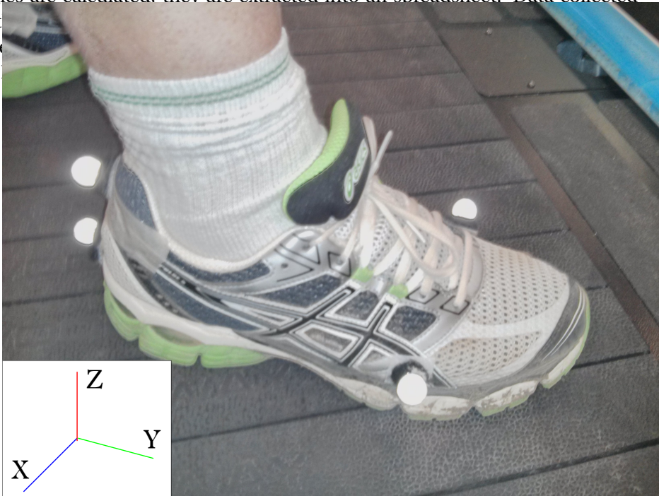
Figure 3.2: Passive markers placed on the shoe. The markers are located at 1 st and 5 th metatarsal heads, and in upper and lower calcaneus
