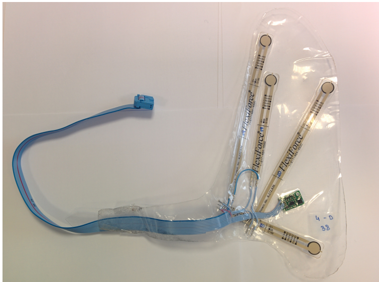
Figure 2.28: Instrumented insole ECnsole version 1.5 showing the four pressure sensors, the IMU (the small green board at the arch of the foot) and the inter-connection wire.
