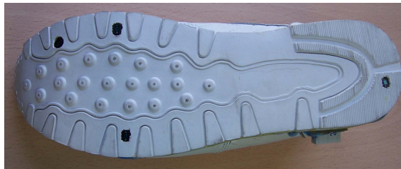
(a) Sole of the sport shoe including photodetectors.
