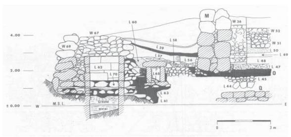
Figure 41: North-south section of the western part of south quay at Dor (Raban 1995b).
