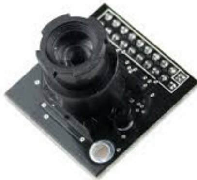
Figure 4.20 – Photo of Camera OV7660 board [34]
