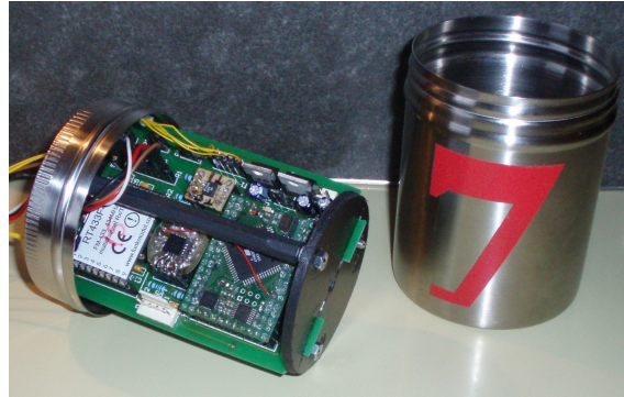
Figure 2.2 – Example of a CanSat [2]
