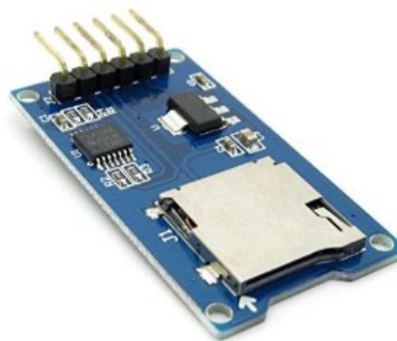
Figure 4.51 – Photo of test board of MicroSD Card Adapter
