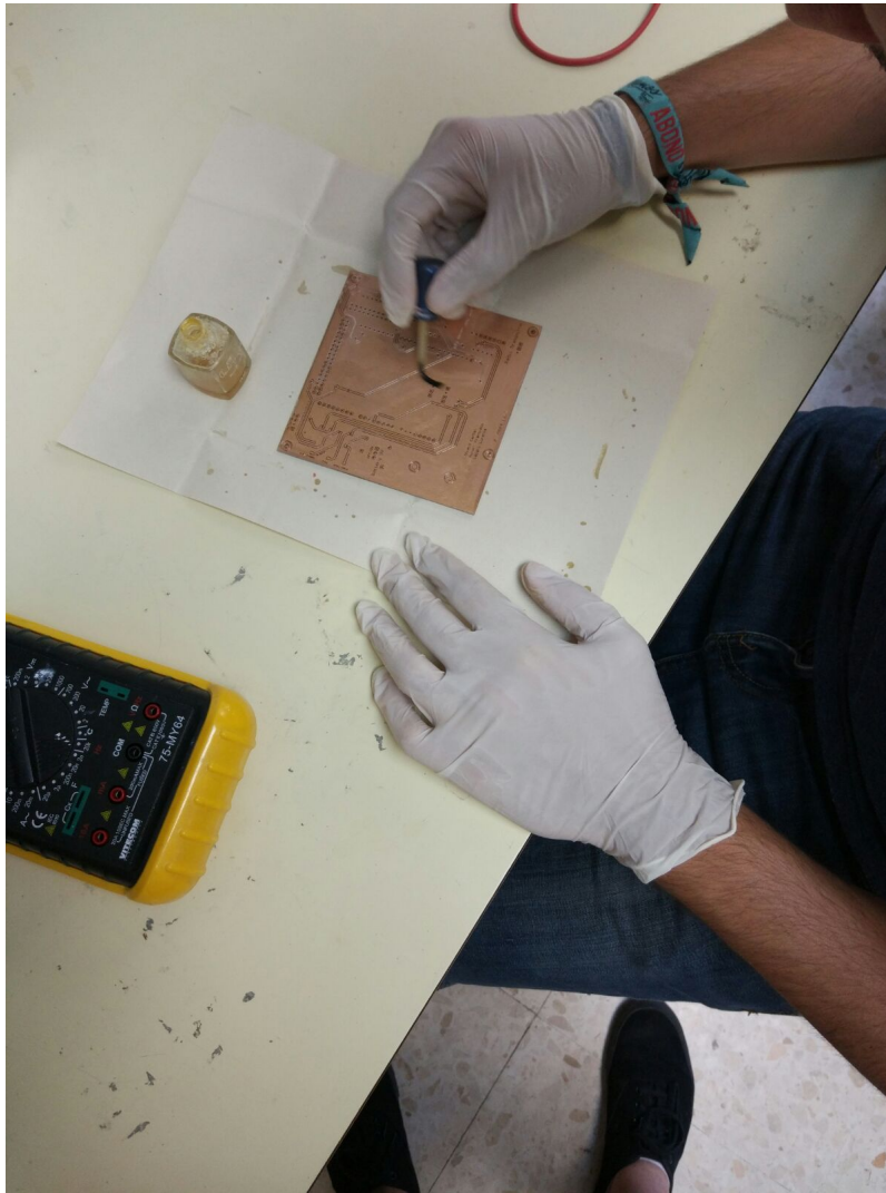
Figure 4.42 – Disassemble Shield CanSat PCB
