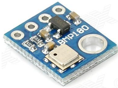
Figure 4.11 – Photo of the test board for BMP180 [7]
