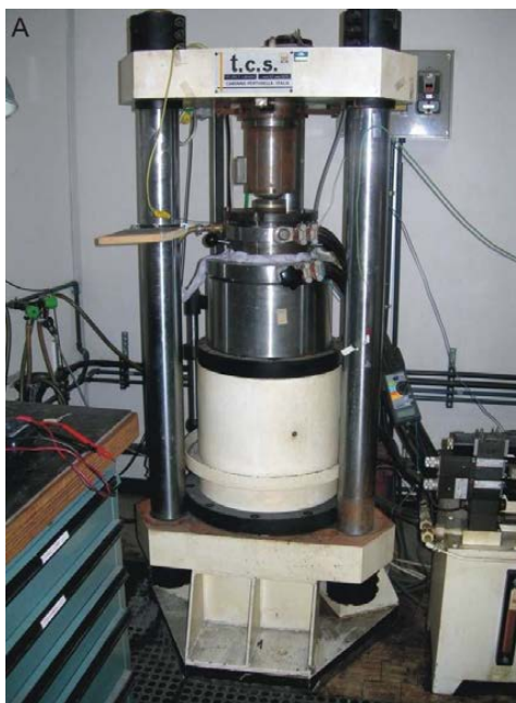
Figure 3.10. Piston cylinder apparatus used for remelting experiments of partially crystallized and nanogranite inclusions (source: Bartoli, 2012)
