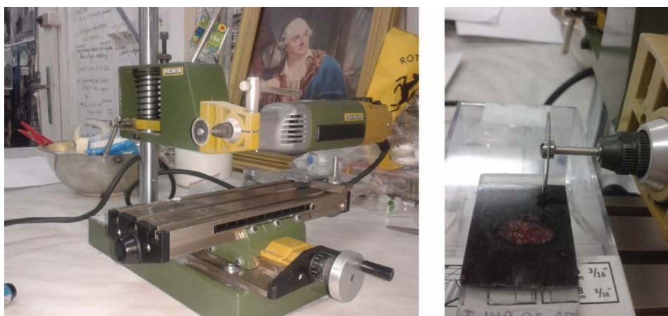
Figure 3.6. Cutting stage for the cutting and mechanical separation of garnet porphyroclasts and porphyroblasts and their cores/rims in thick sections. Diamond saw device (left), and a Jubrique garnet gneiss thick section ready to be cut for separation of garnet cores and rims from the gneiss matrix (right).
