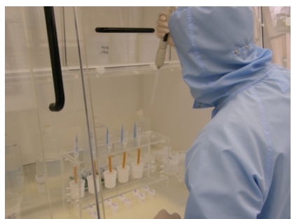
Figure 3.8. Ultra-clean chemistry lab of the Institute of Geological Sciences in Krakow, Poland. (Top) Ultraclean lab with Picotrace® horizontal laminar flow cabinets; (middle) Graphite-Teflon hot plate with Savillex® beakers containing acid digested samples; (Bottom) Operator working with chromatographic columns for separation of Lu-Hf isotopes (top and bottom images from ; http://www.ing.pan.pl/Labs/Lab_GEO-IZO-GEO/Lab_Geo_Izo.htm ).
