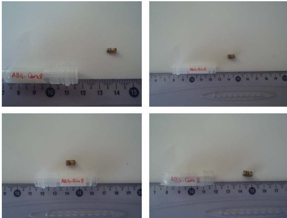
Figure 3.11. Au capsules containing garnet chips with re-melted nanogranites after high-pressure and high-temperature experiments in the piston cylinder apparatus.
